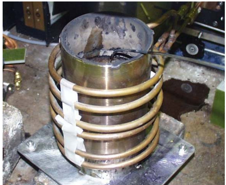
Heating steel crucible for a melting application
