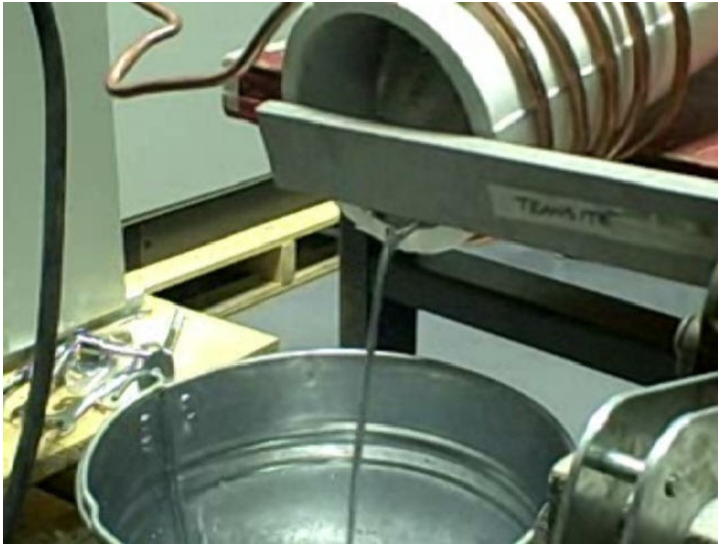
Melted lead pouring from ceramic tube
