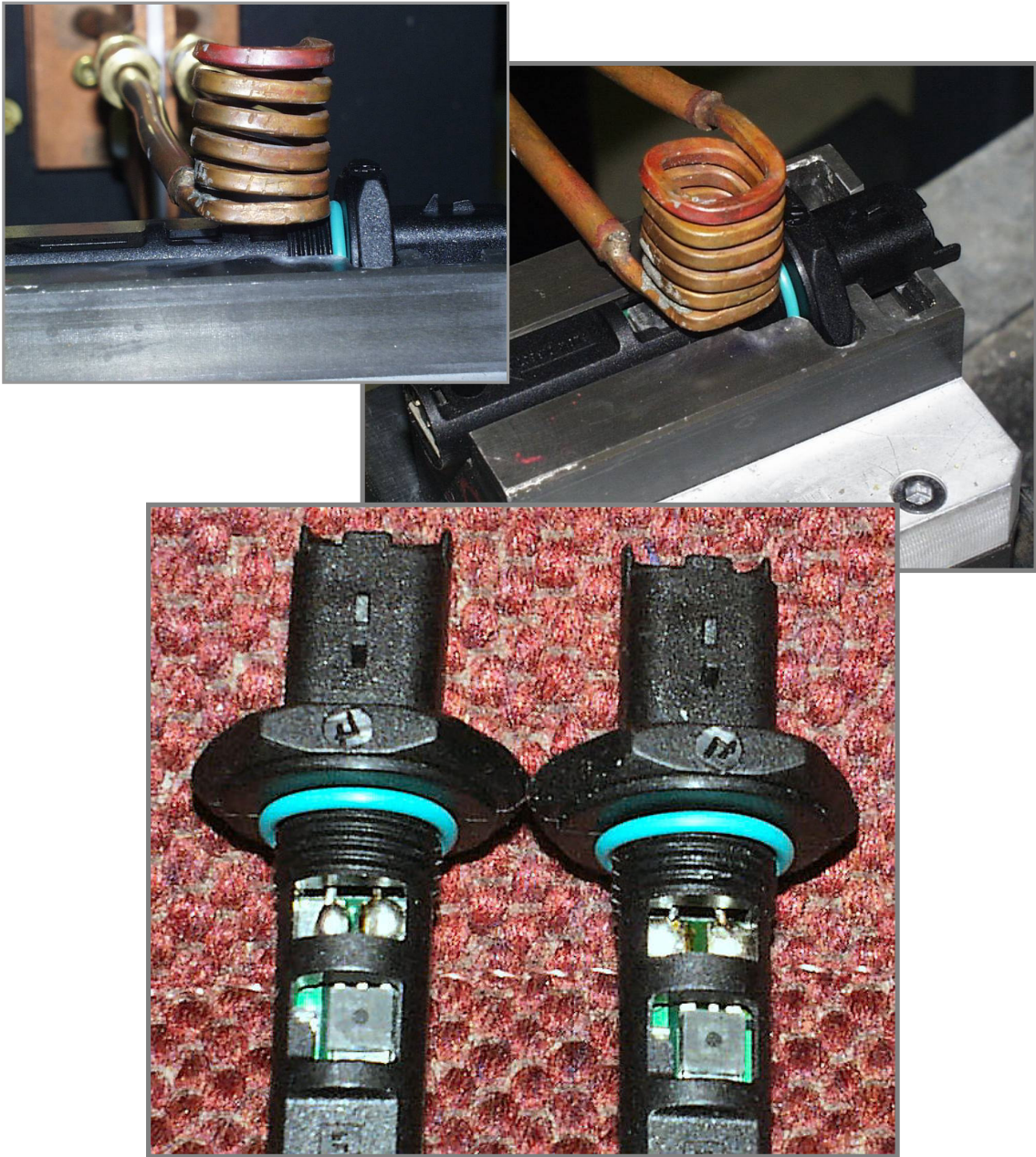
Left – part before solder reflow, Right – part after.
