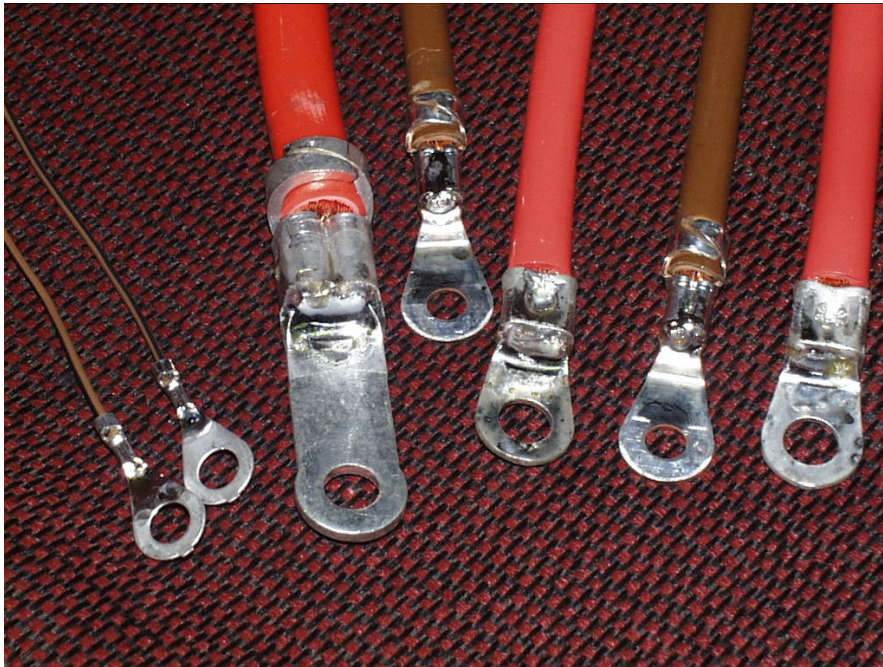
Assemblies of various sizes soldered by the EASYHEAT.
