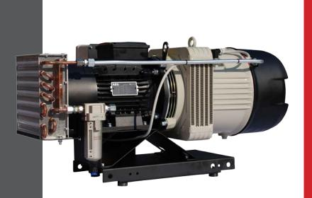
The open frame ERC compressors are used in many different industries, including energy, manufacturing and automotive sectors. The machines are available assembled on a base or air tank with outputs of from 1.5 kW up to 55 kW. They are delivered complete with air cooler, separator and electronic condensation discharger. Their low noise level also means they can be used in stations without a soundproofing canopy.
