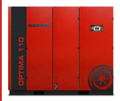
It is a variable speed machine that, owing to its characteristics, is perfectly adapted for the production needs of NolanGroup. Optima 110 comes into play when the production is at full capacity to ensure the correct operation of the factory. The inverter automatically adjusts the rotational speed according to the load profile, ensuring that the air delivered by the system corresponds to the actual demands."
