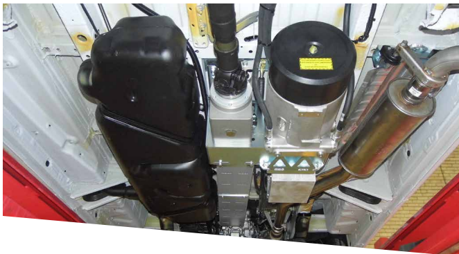
Before (from the top) and After - the underfloor air-compressor (here without generator) mounted to a Thermo King Berlin Transportkälte GmbH vehicle.
