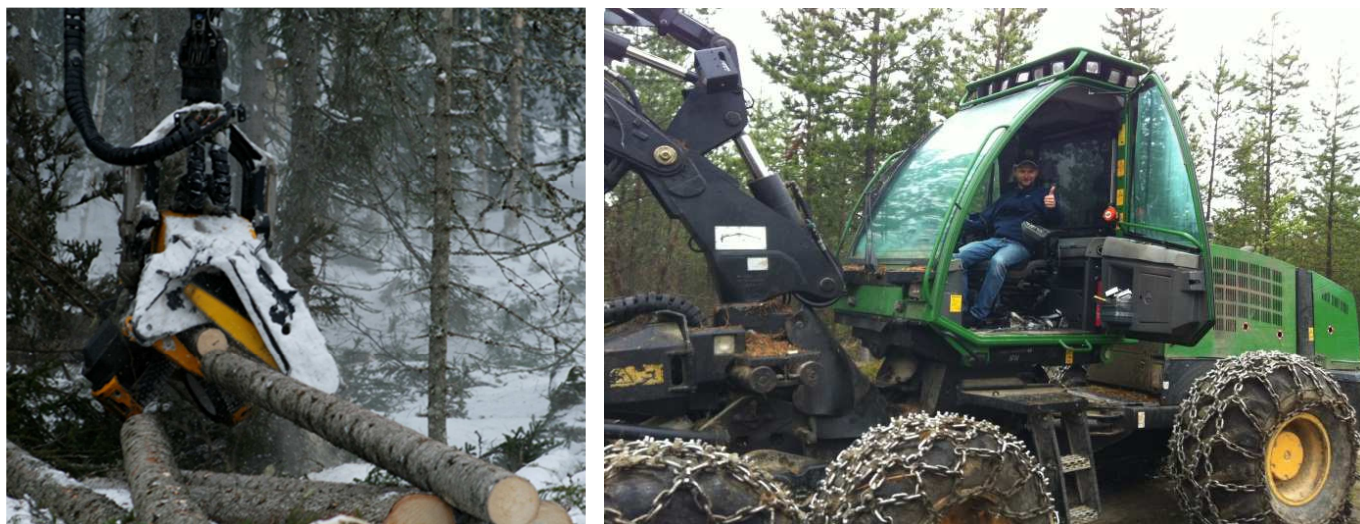
Figure 13: Left: The saw chain in a harvester lubricated with Ca-Bio. Right: Forestry machine where Ca-Bio is used as a general lubricant.
