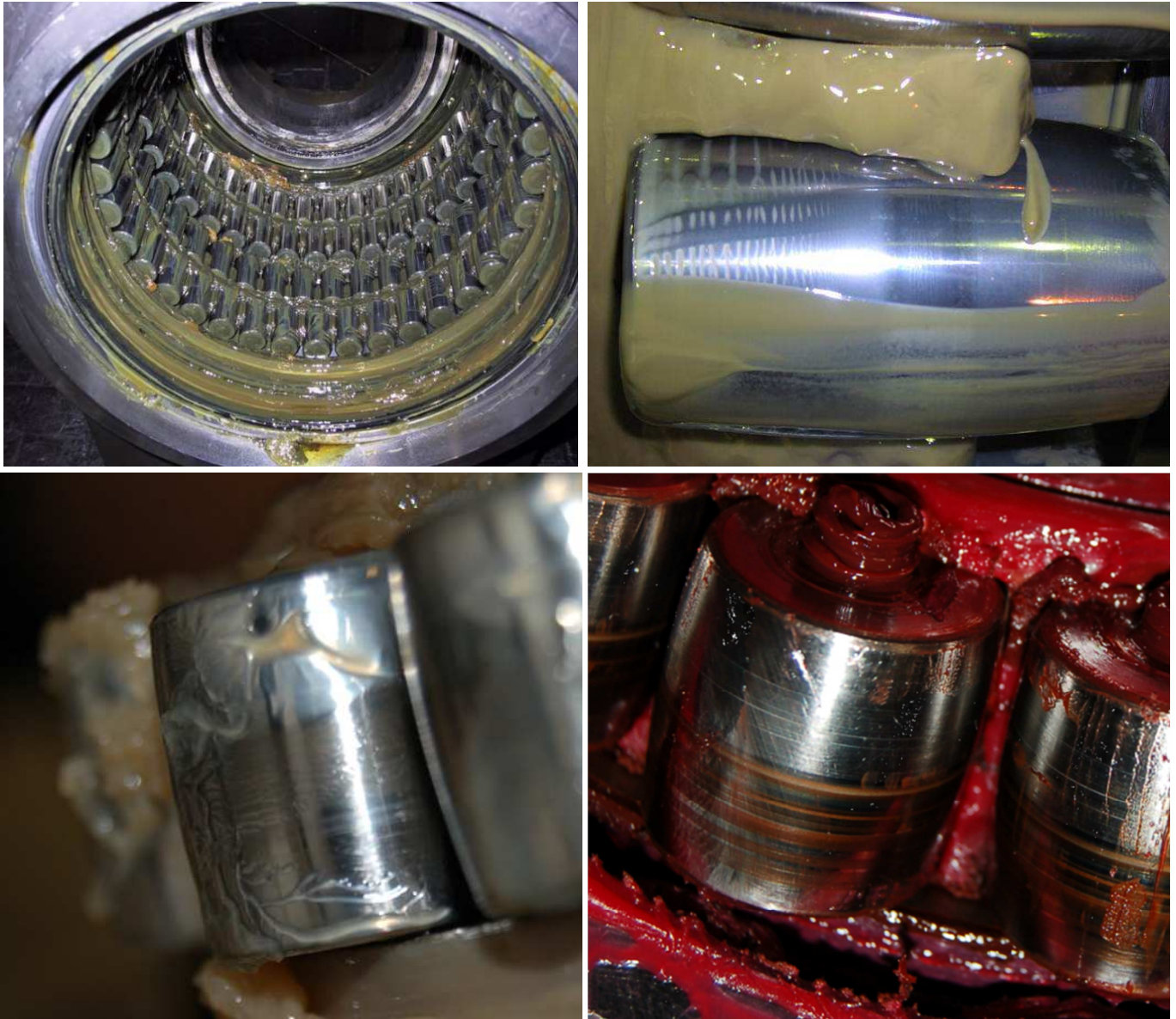
Figure 14: Top left: The bearing from a steel rolling mill disassembled after four shifts without relubrication. Normally lubrication is required several times per shift. Top right: In an aluminium rolling mill the PP grease softened less than the reference calcium sulphonate grease used. In addition, the problem with calcium ions staining the aluminium profiles was solved. Bottom left: The polymer grease used in the wire section of a paper machine where the reference lithium complex grease ( bottom right ) struggled with dry running.
