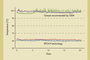
Powertrain has succeeded in reducing the bearing temperature of the flue gas fan by an additional 10 C°, down to an operating temperature of 60°C and this trial will continue until mid-2012.
