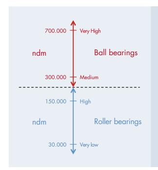
There is unfortunately no standardised way of correlating the speed factor with the structure of the various types of lubricating grease so, for the moment, it can only function as a guideline. The calculation models commonly used only take the base oil viscosity into account and not the thickener type nor the amount. In reality, this will result in a thicker lubricating film than calculated.
