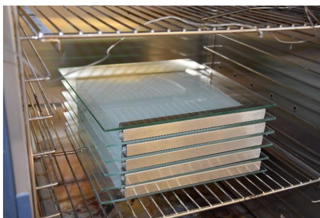
Figure 1: The setup with glass plates used to thermally age the greases
