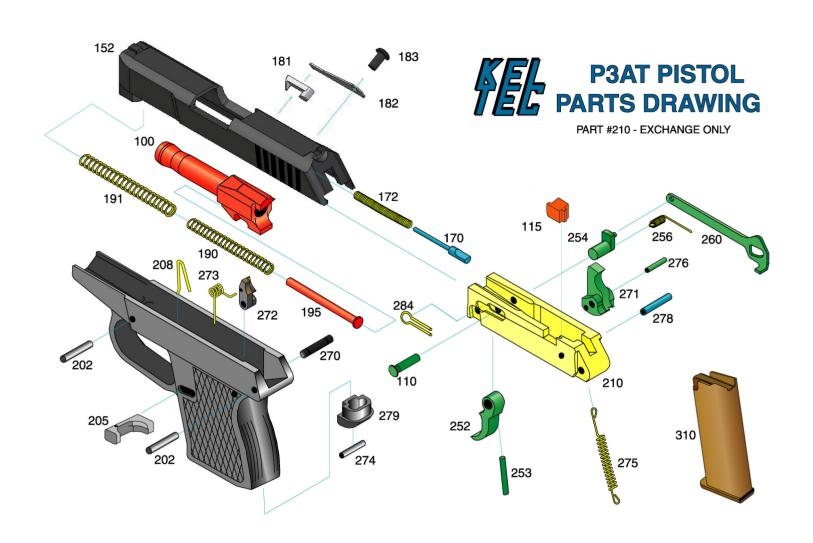
110 ASSEMBLY PIN 115 EJECTOR 152 SLIDE 170 FIRING PIN 172 FIRING PIN SPRING
