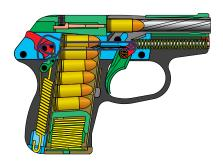
The ignited powder gas drives the bullet forward through the barrel and simultaneously drives the slide and barrel backwards. After about 1/4" (6 mm) the barrel is unlocked by the assembly pin and releases the slide to travel back extracting the case. On it's way back, the slide is gradually slowed down by the recoil springs.
