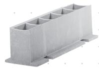
ProTek Composite Pipe Shoe is a UV-resistant, non-metallic solution for elevated or insulated piping systems at the support points. It has 150,000 lbs. of compressive strength, a temperature range of -320°F to +400°F and is resistant to chemical attack. It is the optimal support for insulated or elevated piping systems in plants or refineries, both onshore and offshore.
