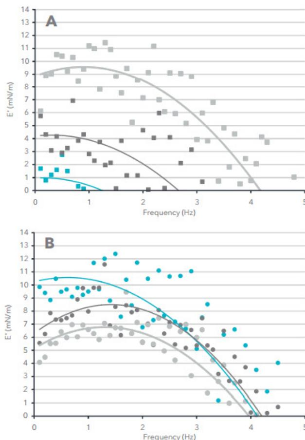
**[Figure 4]:** Change of dilatational elasticity with increasing oscillation frequency in presence of increasing concentration of NF 240 (A) and DF 250 (B). The used concentrations are 8ppm (blue), 25ppm (dark grey) and 100ppm (light grey).
