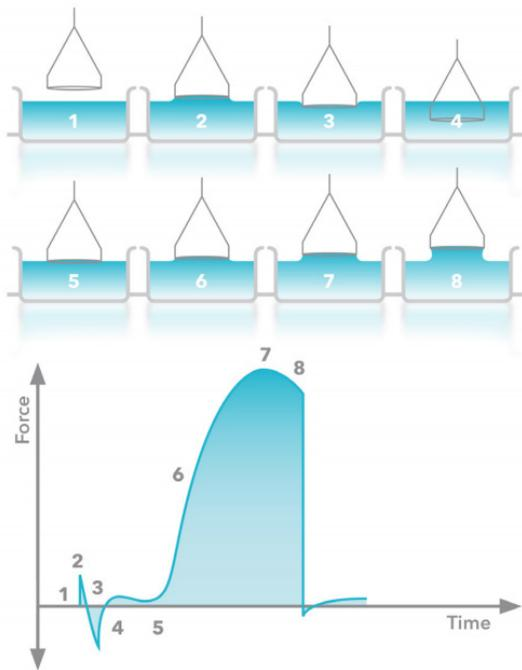
[Figure 2]: Surface tension measurement by Du Noüy ring
