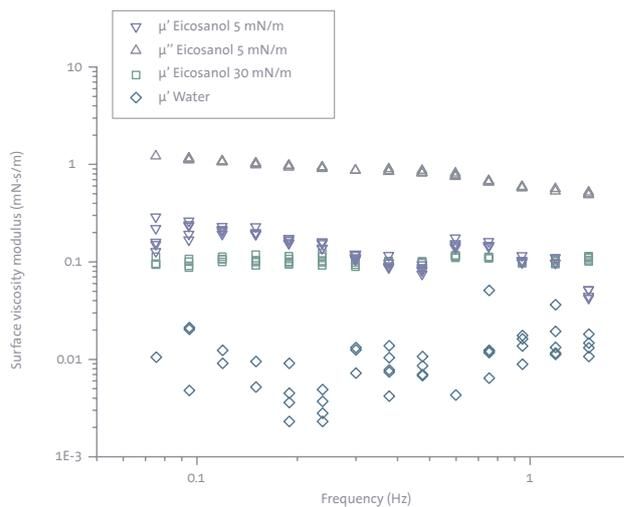
[Figure 4]: Shear rate - corrected surface modulus as a function of frequency for eicosanol at 5 mN/m, 30 mN/m pressure and for pure water.  $\mu''$  for eicosanol at 30 mN/m and water is not seen in the figure.
