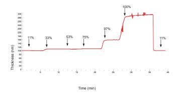
[Figure 2]: Thickness of NPS as a function of air humidity.
