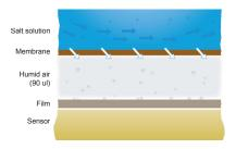
[Figure 1]: The Q-Sense Humidity Module in cross-section.
