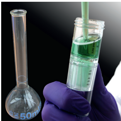
[Figure 1]: Illustration of equipment in which borosilicate and PVDF is used: a volumetric flask and a protein spin concentrator.
