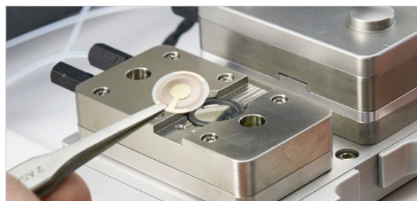
Temperature controlled environment for sensor and sample
