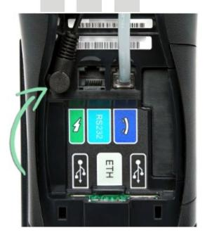
5. Plug the power adapter into a power outlet. This will turn the terminal on automatically.
