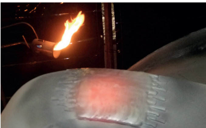
Figure 9: First completed section of as-welded stabiliser using Colmonoy® 25F
