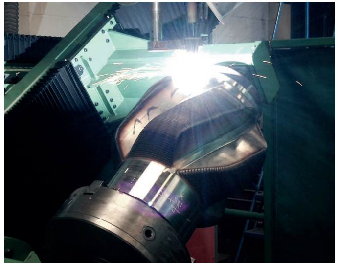
Figure 2: PTA Machine applying coating to a downhole tool Photo courtesy of Lion Engineering Ltd (Great Yarmouth)
