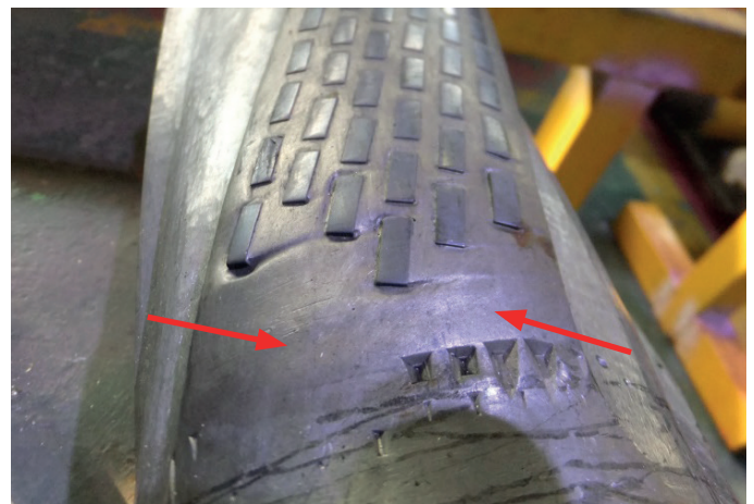
Figure 10: Image shows the leading edge with tile loss and erosion of the cementing matrix powder. Further use would result in rapid tile loss. Colmonoy® 7541-55F improves performance in reducing wear rates in this area
