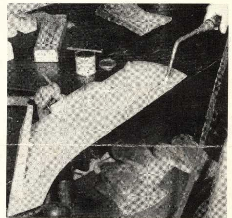
Figure 2 . . . MOLDBOARD bottom blades protected with Wall Colmonoy hard-facing alloys. Upper share has plowed in excess of 1400 acres at Wood River, Nebraska; edge is still sharp and in good enough condition for plowing an additional estimated 1000 acres. Lower blade was hard-faced when new—has plowed more than 1600 acres—is still in excellent condition. These useful life figures compare with a normal useful life of 30 to 60 acres for an unprotected share in the Wood River area soil.
