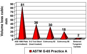
The chart compares abrasive wear test results of several materials under the same conditions. The relatively low volume loss proves the superiority of Colmonoy 88 to all but the hardest of materials.
