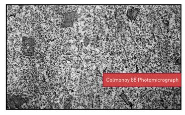
As an integral part of Colmonoy<sup>®</sup> 88 alloy, these hard phases do not sink or settle out during the application process as would the carbides in a blended composite powder. Thus, the first 0.001" layer and the last 0.001" layer are virtually the same.
