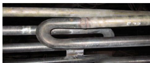
Figure 2: Colmonoy 88 Spray & Fuse overlay protecting Inconel tubes in core of Super heater boiler [4]
