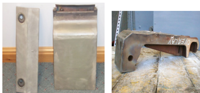
Figure 6: Colmonoy 88 coated side plates and grate bar casting
