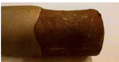
Figure 5: Super heater tube showing coated and uncoated areas after 8000h service [2]
