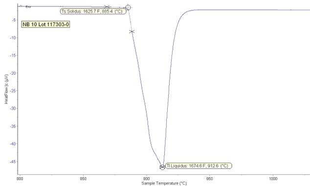
Figure 3a shows a DSC chart for Nicrobraz® 10 (BNi-6) with 11.33% Phosphorous and indicating slightly incongruent melting.
