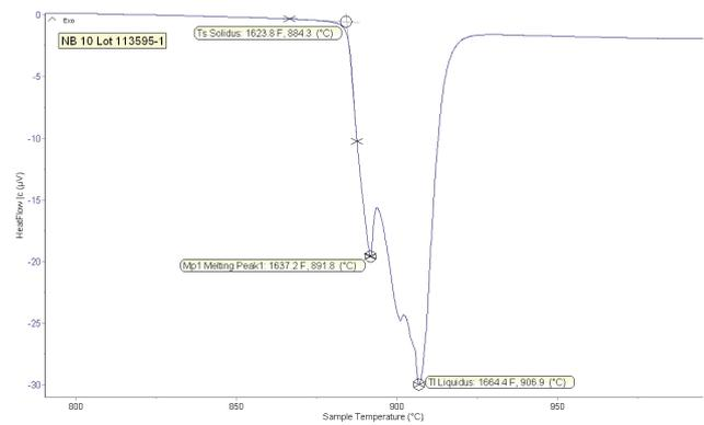
Figure 3c shows a DSC chart for Nicrobraz® 10 (BNi-6) with 10.16% Phosphorous and indicating incongruent melting.
