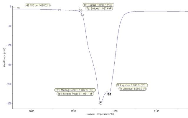
Figure 2. shows thermal analysis results, also for Nicrobraz® 150 (BNi-9) following EN 3877 method modified for Differential Scanning Calorimetry (DSC). Heating curve, (10°C/min), temperature versus heat flow, indicates solidus of 1058.7°C and liquidus of 1093.3°C.
