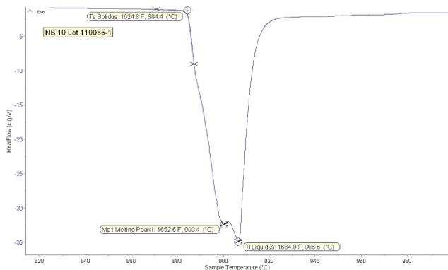
Figure 3b shows a DSC chart for Nicrobraz® 10 (BNi-6) with 10.34% Phosphorous and indicating incongruent melting.
