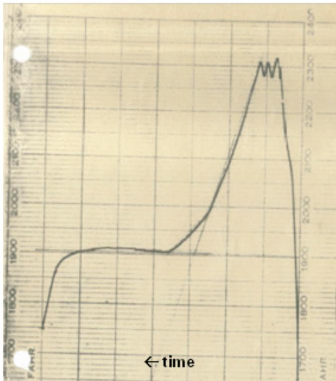
Figure 1. Cooling curve for Nicrobraz® 150 (BNi-9) conducted in April 1956 by Wall Colmonoy Corporation. Cooling rate ~6.5°C/min. Solidus ~1040°C; Liquidus ~1046°C. Photocopy of a scrolling autopen chart recorder where time is increasing from right to left. The temperature spike at the right side indicates initial contact between thermocouple and liquid metal sample.
