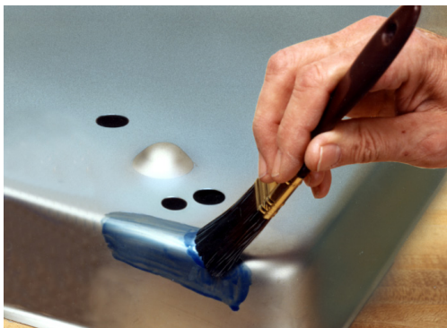
Blue Stop-Off brushed onto surface part
