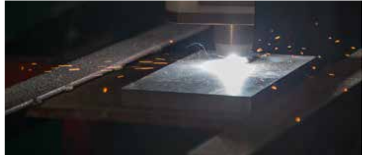
Above: Depositing Wallex 6 PTA: WCL (UK) Aerobrazed Facility
