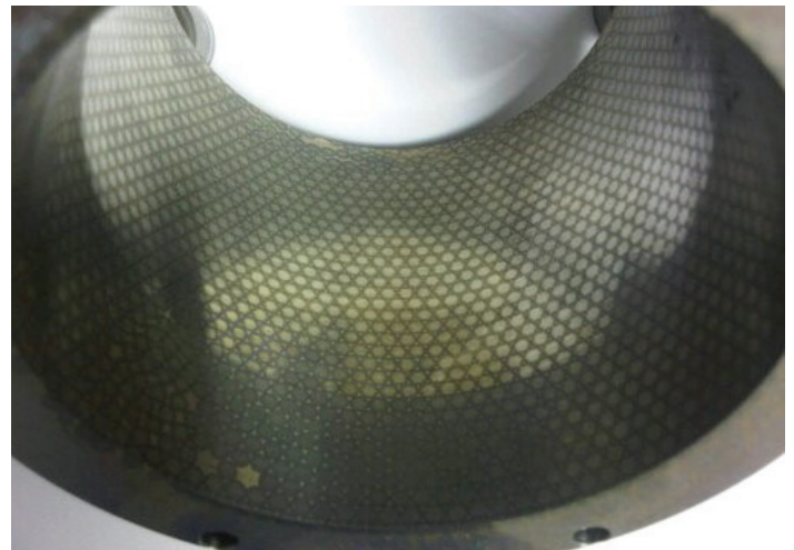
Bearing with WallCarb™ coating inside
