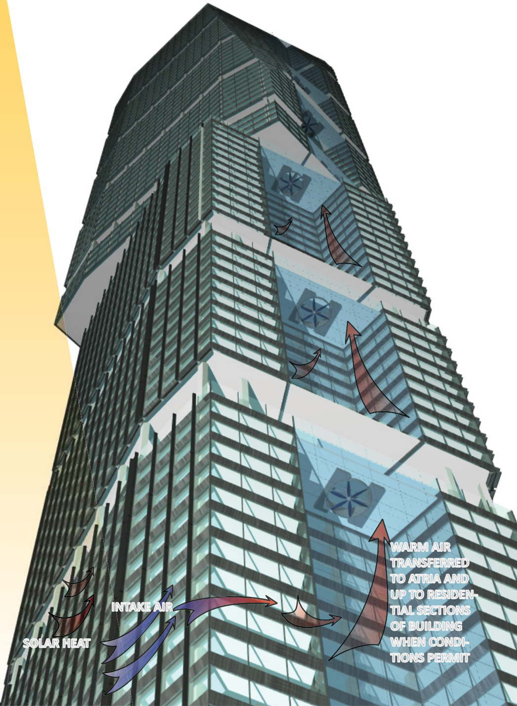
4 MECHANICAL DIAGRAM UTILIZATION OF THE EXISTING MECHANICAL SYSTEM ON THE EXISTING COMMERCIAL FLOORS, NEW MECHANICAL SYSTEM FOR THE PROPOSED RESIDENTIAL SECTION OF THE BUILDING.
