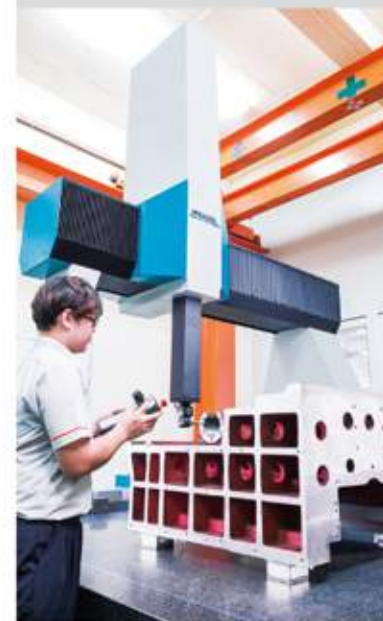
CMM accuracy inspection of components
