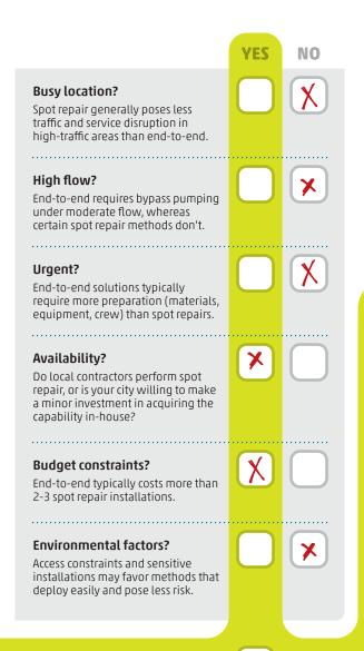
A range of technologies are available to repair any sewer pipe. Choosing one means first determining whether end-to-end (manhole-to-manhole) or spot (point) repair is advised. Here we present 12 of the most important considerations. Simply tabulate your "yes" answers in each column to understand where a given pipe falls on the recommendation matrix.
