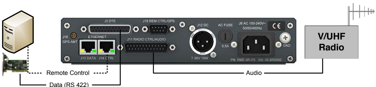
Figure 1: RM8 based Synchronous V/UHF Data System
