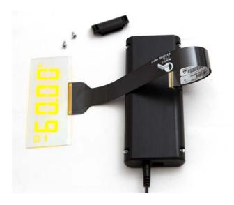
Lamination Introduction Package (LIP) ELT40S-07 is a bundle of TASEL<sup>®</sup> display panels (Lumineq ELT40S TASEL display), flexible printed circuit (FPC) cables and driving electronics. With the product, Lumineq customers can experiment with various levels of display in-glass lamination.
