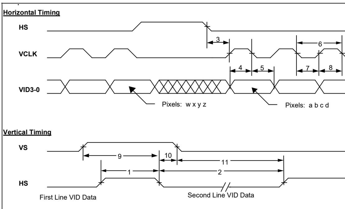
**Figure 2. Video input timing diagram**
