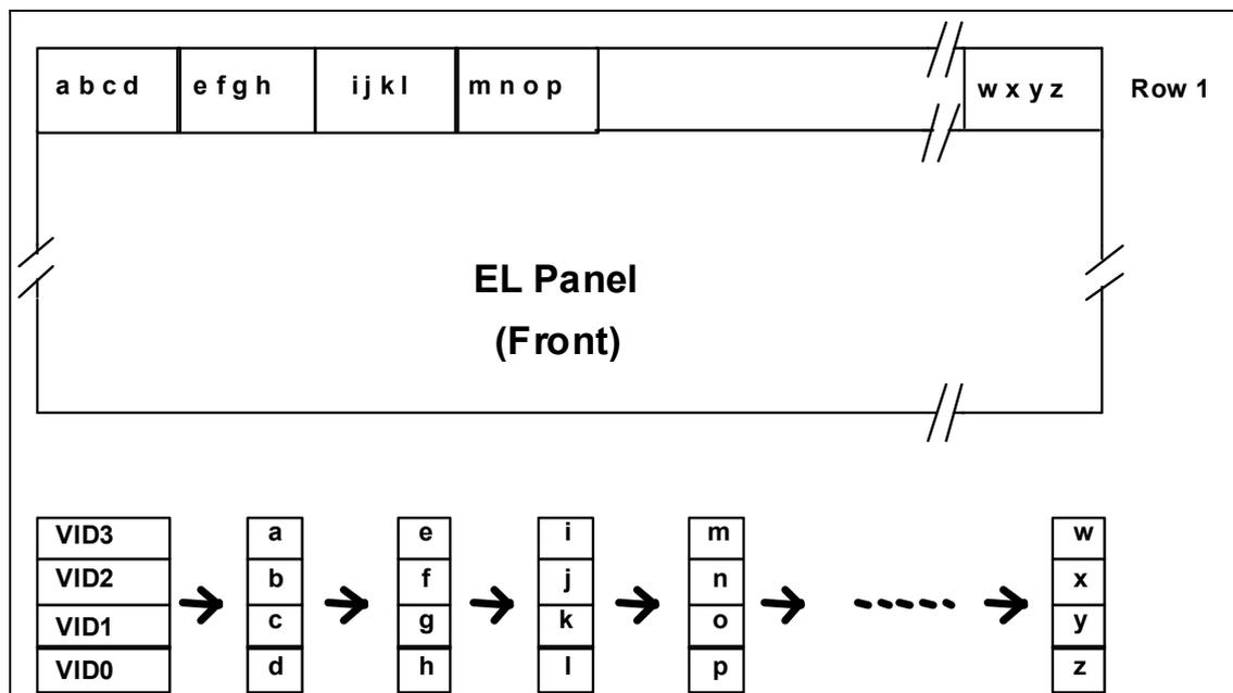
**Figure 3. Pixel location versus sequence of data**
