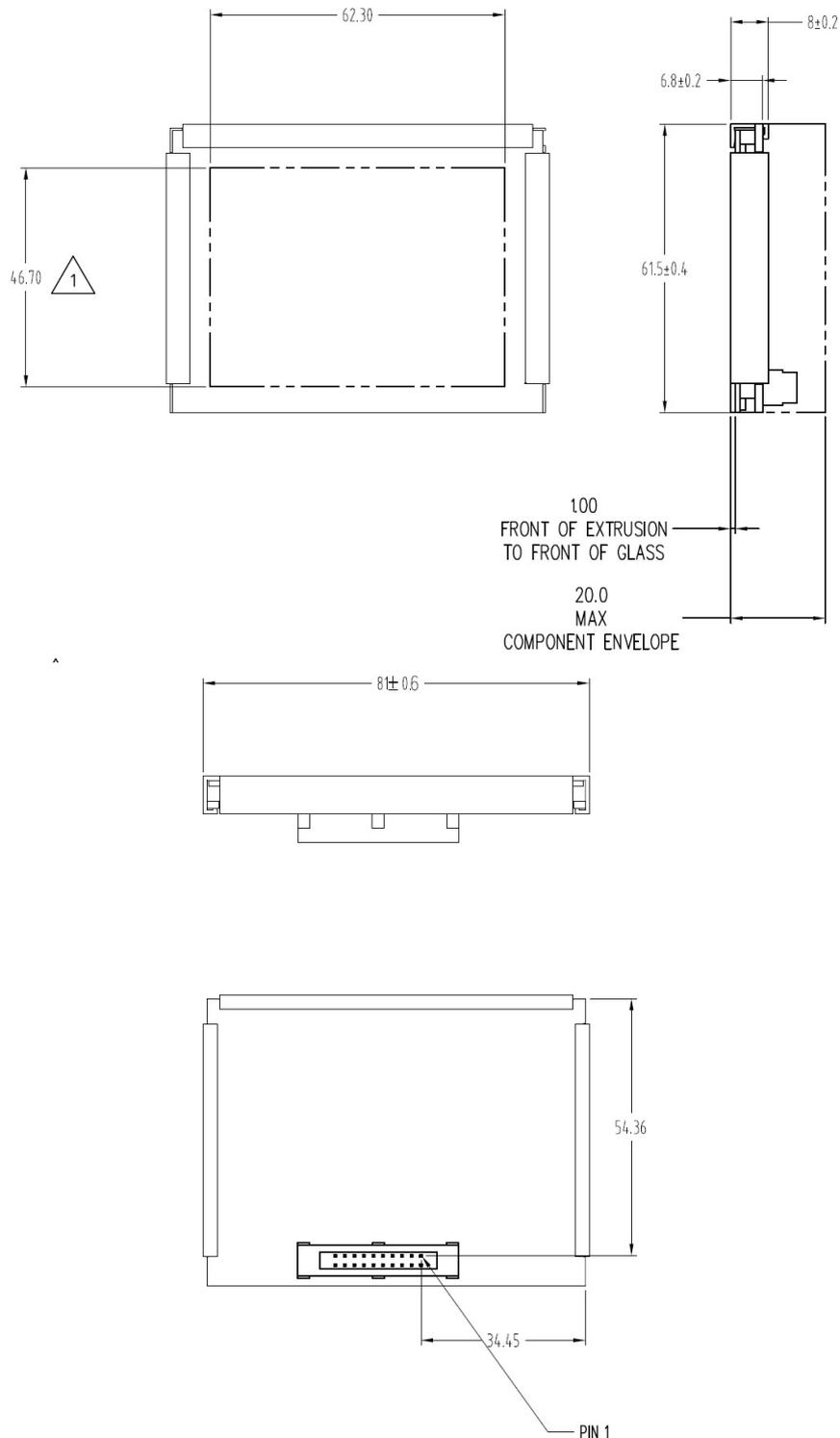
**Figure 5. EL160.120.39-NE display dimensions**
