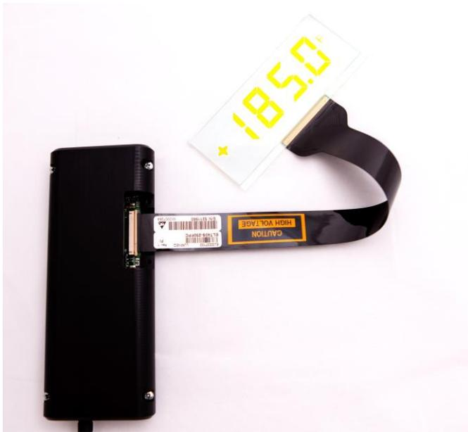
TASEL Introduction Package (TIP) ELT40S is a bundle of one TASEL® display panel (Lumineq ELT40S TASEL display), flexible printed circuit (FPC) cable and driving electronics.
