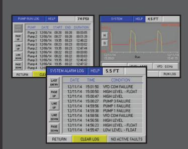
The PV600 records operating conditions with data logs and trend charts that are viewable on the controller screen and are stored on an SD card for permanent record. Separate logs exist for system faults, pump faults, and pump run times. Trend charts are provided for level, pressure, flow, VFD speed, number of pumps running, and temperature.
