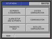
Setting the PV600 up to your unique application is simple due to the easy and intuitive menu structure that is accessed through a three tier security system. All parameters, such as type of starters or VFD, sensor types and ranges, set points, sequencing, communications and more, are easy to find and modify without referring to a manual.
