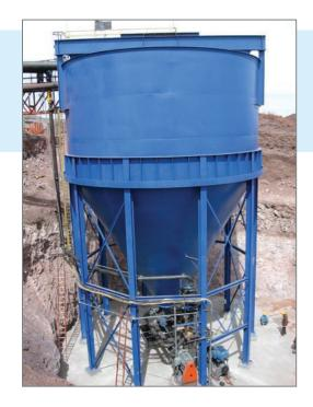
The AltaFlo<sup>TM</sup> ultra high-rate thickener is a rake-less thickener that provides mixing, flocculation and internal dilution, followed by clarification and positive sludge collection and removal, all in a single tank. The principles of dewatering have been further optimized to a new design that thickens slurries at an even higher rate than a typical high-rate thickener.
