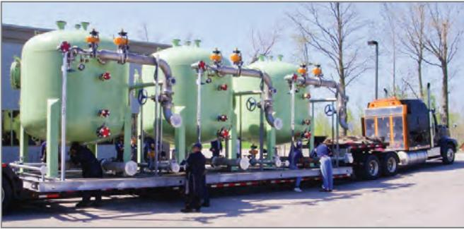
For nearly half a century, WesTech has been a recognized leader in the manufacture of granular activated carbon (GAC) contactors for municipal and industrial water treatment. Choosing a GAC integrator with complete process knowledge and years of water treatment experience is a vital part of your GAC solution.
