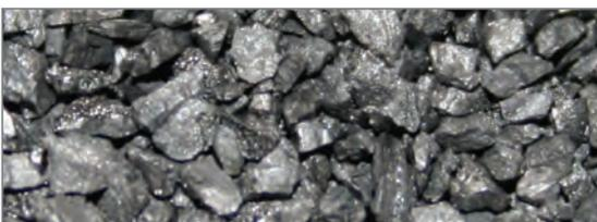
**Granular Activated Carbon:** Commonly used for adsorption applications, e.g., taste, odor, TOC, SOC removal.
