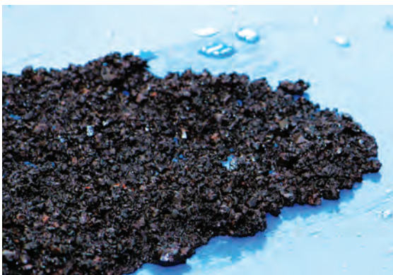
Granular Ferric Hydroxide: optimized for arsenic and other heavy metal adsorption applications.
