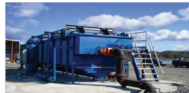
Rectangular tanks are easier to install while circular DAF designs require less maintenance
