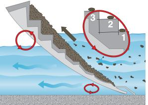
The blades in the lower part of the unit move in an elliptical horizontal motion, while the blades in the upper section move in the traditional circular motion. This progressive motion moves the captured solids (precoat solids) up the screen at a slower and more even rate.
