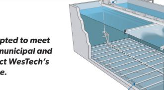
Sludge Scraper Wedge Sections and HDPE Strips
