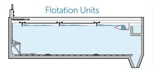
The effectiveness of the ZICKERT Scum Skimmer has proven to be a simple and reliable solution for dissolved gas flotation units and oil/water separators. The adjustable skimmer and float box provide the flexibility for solids removal. The ZICKERT Shark can be applied to pretreatment, thickening, or refinery processes.
