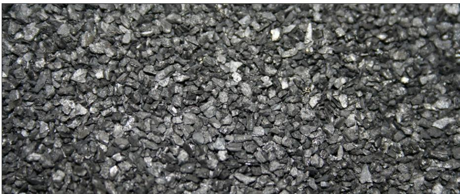
**Granular Activated Carbon** is commonly used for adsorption applications, e.g., taste, odor, TOC, SOC removal.
