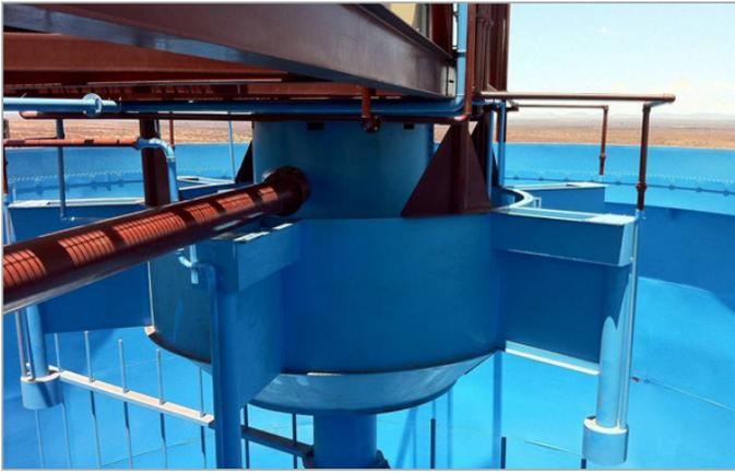
WesTech's **AirLift™ Dilution System** uses an airlift pump to draw clarified water evenly from the thickener surface into the feedwell. An even draw from multiple points prevents flow disturbances in the quiescent settling zone while ensuring proper dilution and feed mixing inside the feedwell. Dilution flow can be regulated with precision by operator adjustment of the airflow to the system.
