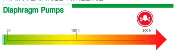
After every 300 hours or at season's end (whichever comes first) install a new set of diaphragms flush valves. and with clean water before and inspect Always drain pump servicing or disassembling. For complete service instructions, please refer to Comet literature. We suggest to use only Comet original Spare parts.
