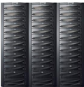
The enterprise-class CX3 model 80 shares the same hardware and software architecture as the CX3 model 40 and CX3 model 20, but with faster processors, higher capacity, greater connectivity, and greater throughput. It scales from 5 to 480 disk drives and supports up to 256 dual-connected hosts.
