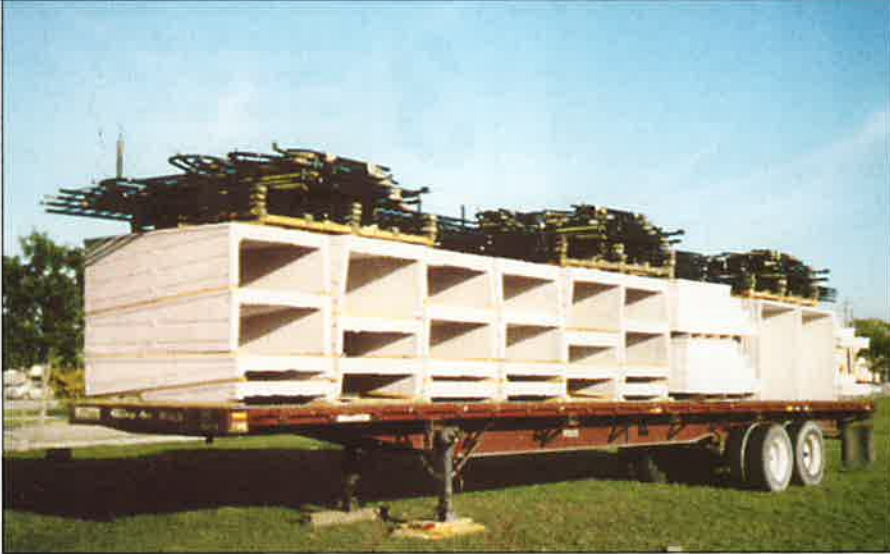
Six complete Access Systems, their hollow components neatly stacked, fit on one flatbed for delivery.
