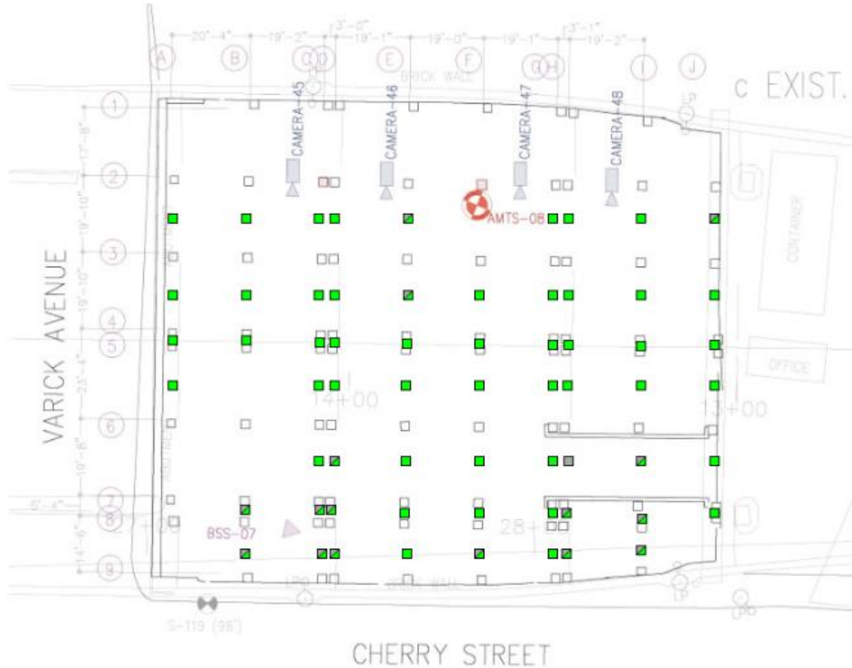
Figure 6. Typical Differential Settlement Monitoring Plan of Brooklyn Connector between Varick and Stewart Avenues
