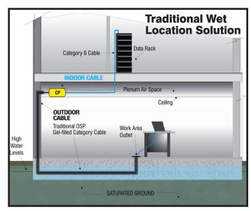
Outdoor (non-rated) cables are often used for below grade and in-the-slab applications. In these instances, the outdoor cable must transition to the appropriately rated indoor cable, such as plenum or riser, upon entering the building interior. This method of using two types of cable requires additional materials and labor as well as space for the consolidation point.
