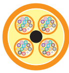
48-fibers (4 tubes of 12-fibers)
