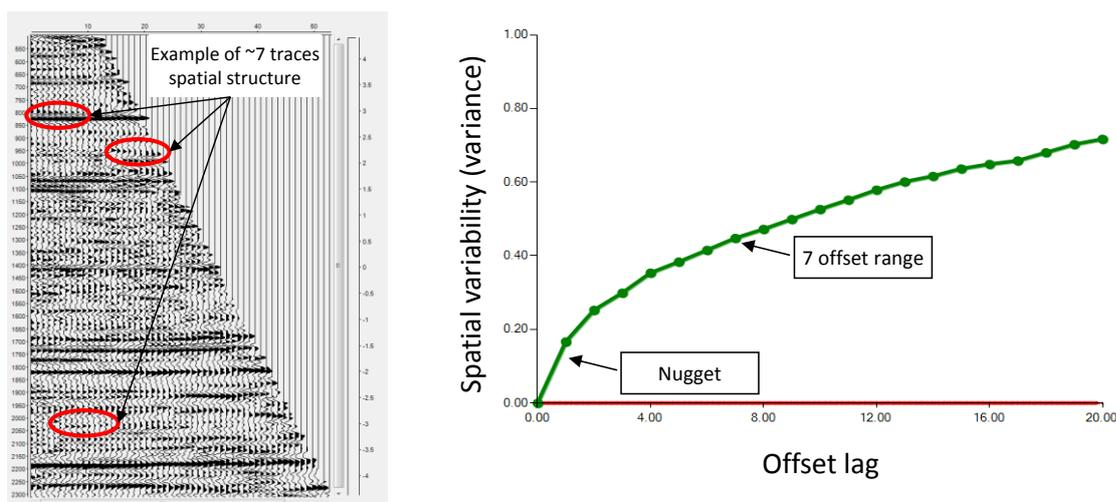
**Figure 1** Interpretation of variogram of a pre stack gather in the offset direction in terms of noise non correlated from trace to trace (nugget component, noise correlated from trace to trace (short 7 offset range component) and signal (long spatial range > 20 offsets component)
