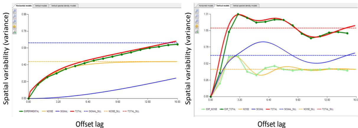
**Figure 2** Modelling experimental variograms (green lines) with red curve of in the offset (left) and time (right) direction in terms of noise correlated and non-correlated from trace to trace (brown curve) and signal (blue curve)
