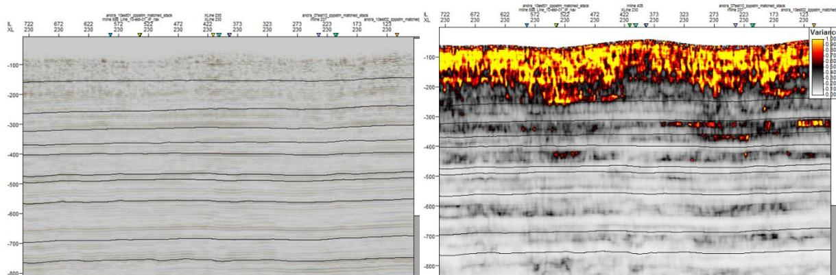
**Figure 3:** Stacked amplitude section (left) and SQI indicator of the reliability of the stacked amplitude values (right). White SQI areas (near 0% error) indicate reliable amplitude values. Dark to red SQI areas (above 50% error) indicate non reliable amplitude values. Horizons (black lines) interpreted on the stacked section (left) can be checked on the SQI section (right)
