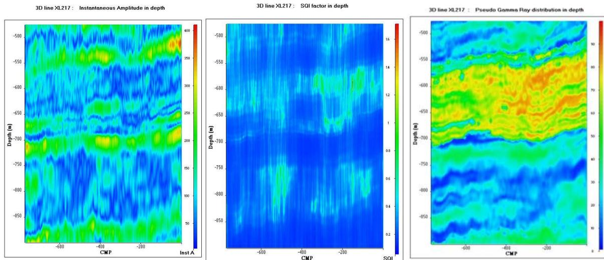
**Figure 3:** Instantaneous amplitude (left), SQI factor (center), and pseudo gamma ray distribution in depth.
