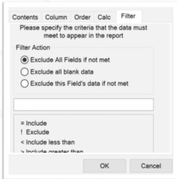
This allows “selective” rule-based reporting. It uses ‘**Boolean**’ filters to qualify data. For example, equals or not equals, less than or greater than. It can filter entire items or only certain fields. For example, display length or angle for certain items but not others. It also can be used to filter objects that don’t appear on the report as a filter. For example, **Item Cut Type = Decoiled Straight**.
